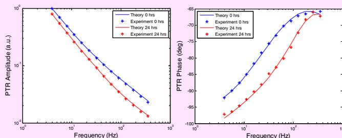
Theoretical 3-Layer diffuse-photon-density-wave and thermal-wave model describes the frequency dependence of the PTR signal (A. Hellen *et al*, Applied Optics 49, 2010).
