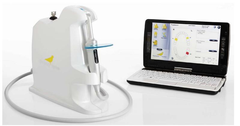
□Pulses of laser light (660 nm) are shone on the tooth and the laser light is converted to four signals during a 5 second scan: 1) The strength of the converted heat (PTR Amplitude); 2) The time delay of the converted heat to reach the surface (PTR Phase); 3)The strength of the converted luminescent light (LUM Amplitude); 4) The time delay of the converted luminescent light (LUM phase).
