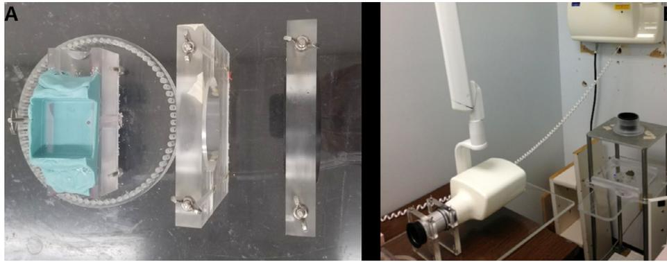
Fig. 4. (A) Fixed base made of Sil-Tech condensation silicone and 2 fixed 2-cm-thick acrylic plates used to stabilize the x-ray tube head and standardize the tooth position during x-ray exposure. (B) Intraoral radiograph acquisition using the Planmeca intraoral dental x-ray machine with the tube head positioned in the experimental setup ready for exposure.
