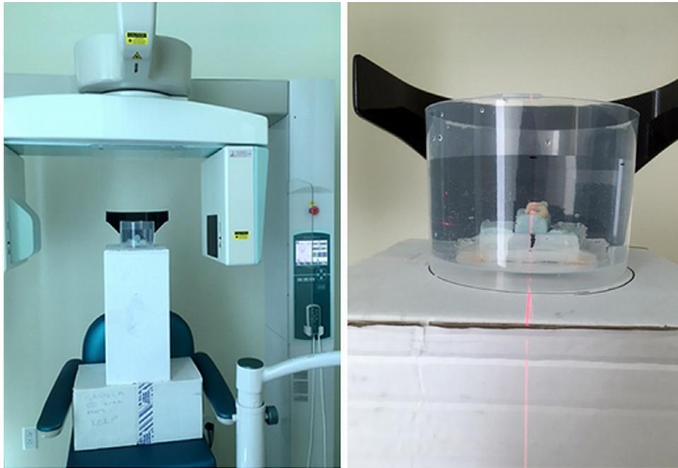
Fig. 6. Cone beam computed tomography (CBCT) acquisition using the 3 DX Accutomo H CBCT unit with teeth placed in a water-filled bowl to simulate soft tissue.
